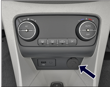
Power Socket Front
