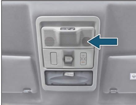
Mic is provided on the roof near the roof lamp.
